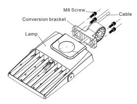
2.The cable passes through the conversion bracket and is fixed conversion bracket to the lamp with M8 screws.
