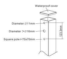
3. Open the waterproof cover of the square pole and confirm the installation hole position on the square pole.
