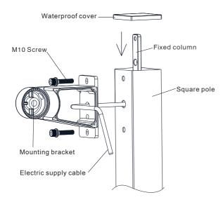
4. The cable passes through the mounting bracket; The mounting bracket is fixed to the pole with M10 screws;
