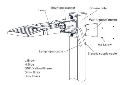
5. The lamp and mounting bracket are reliably fixed, the cable is properly connected and hidden in the mounting bracket cavity. The sealing ring on the bracket cavity, and the waterproof cover is fixed to ensure waterproofing.
